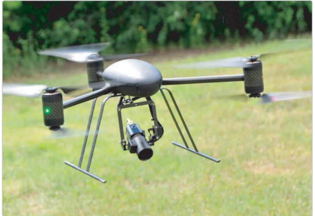
Low Light Video Camera w/ Anti-Vibration Mount & Wireless Video Transmitter
