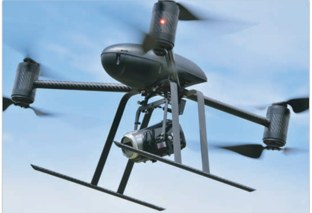
HD Video Camera with Anti-Vibration Mount and Wireless Video Transmitter
