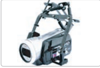
HD Video Camera with Anti-Vibration Mount and Wireless Video Transmitter
