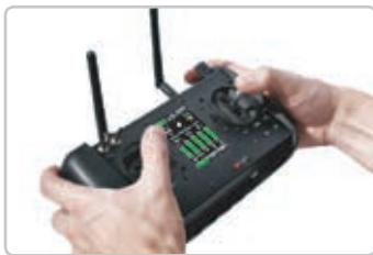
2 Handheld Controllers with Touchscreen Displays and Wireless Video Receivers
