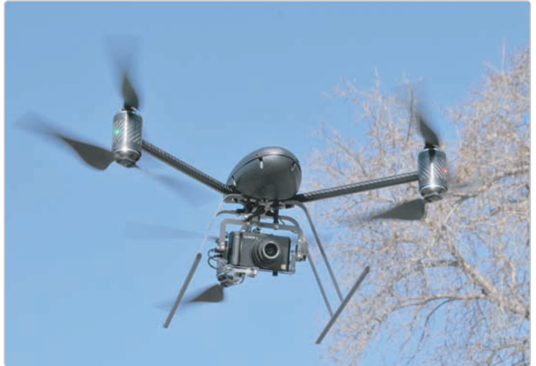
10.1MP Digital Camera with 720p HD Video, Anti-Vibration Mount, and SD Wireless Video Transmitter
